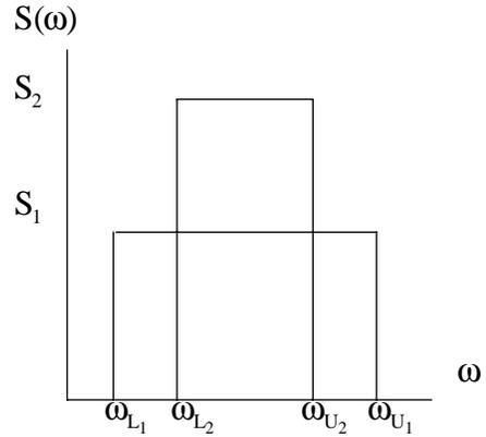
Note that wave damping of these systems depends essentially on the *mean* drift force, which is the same for these two spectra so that *total* dimensionless system damping  $\Gamma$ , *including* wave-drift contribution, is the same for the two cases (damping in percent of critical  $\equiv 50 * \Gamma$ ).
