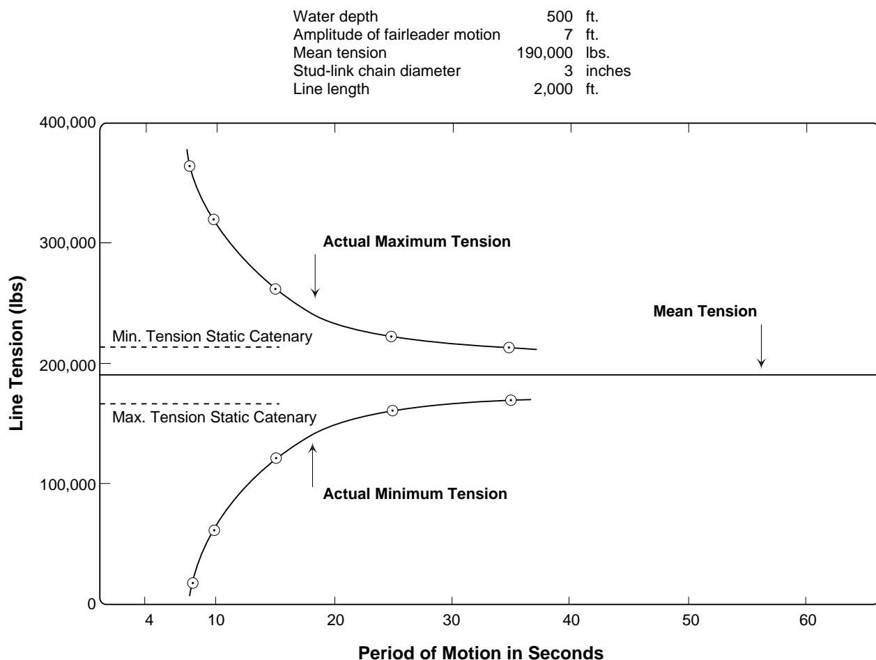
Chain mooring lines can also become slack (or nearly slack) during part of the fairleader motion cycle but a larger motion amplitude is usually required for this to occur. Again, when the fairleader motion is large enough for the line to just go slack the peak tension will be about twice as large as the mean tension. The tension oscillations may be increased by as much as 10 times by the dynamic forces.
